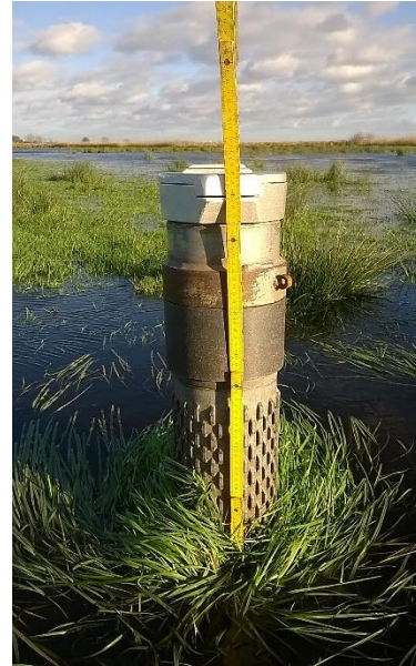
Fig. 2: Groundwater level measuring station (established in 1989) which indicates a loss of height of 1,45 cm/a despite 30 years of ditch blocking and flooding in a nature protection area.
