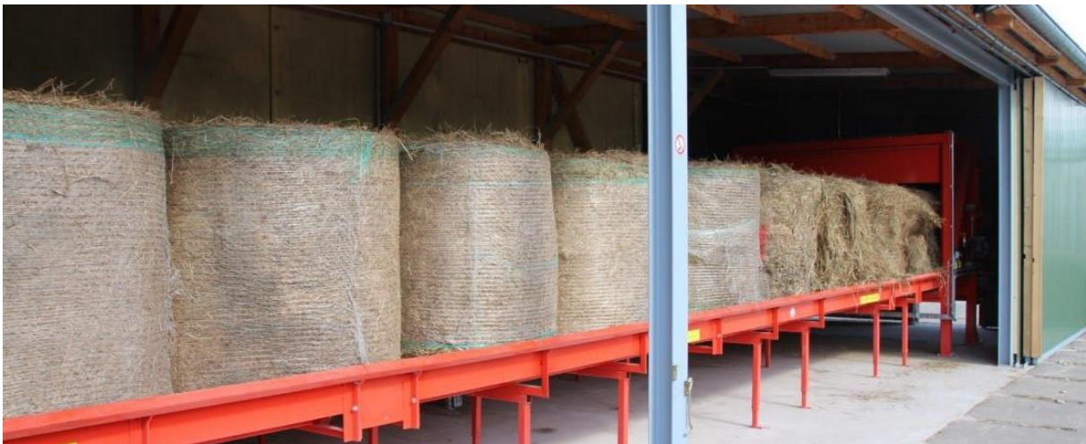
Conveyor and disintegration unit for round bales (W. Wichtmann).
