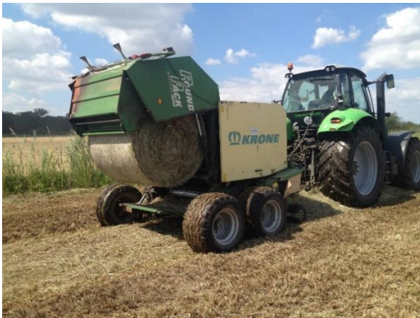
Harvesting Neukalener Wiesen in late July 2018 with adapted machinery (tandem axis, wide tires with low pressure) at groundwater tables of 25 - 35 cm below soil surface.
