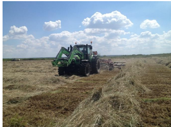
Harvesting Neukalener Wiesen in late July 2018 with adapted machinery (tandem axis, wide tires with low pressure) at groundwater tables of 25 - 35 cm below soil surface.
