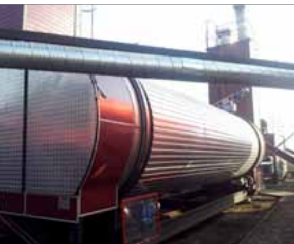
Rotating drying devices at the Mini-briquette factory Lidski near Dokudovskoe, Belarus (S.P.Kundas)
