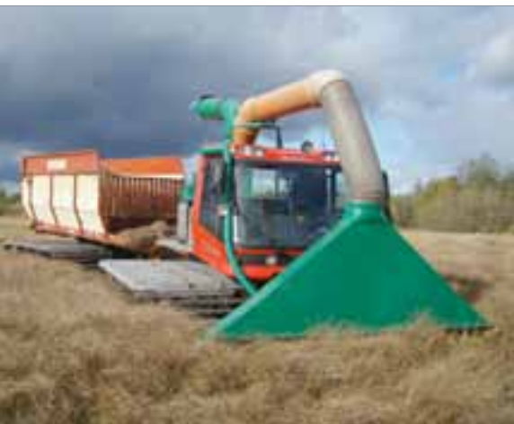
Adapted harvesting system for wet peatlands, based on snowcat (Ratrac) technology can be applied on very wet and soft peatland soils. It minimises mechanical impact on the vegetation and the peat soil surface. Vysokoe, Yaselda lowlands, Belarus (A. Haberl)
