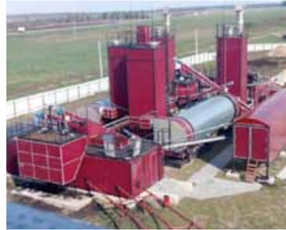
Production unit for manufacturing briquettes from paludiculture biomass. First tests with different mixtures of biomass and peat gave promising results. They showed that 100% biomass briquettes are feasible, make sense and are the only sustainable way to produce regional fuels so far (V.N.Potupchik)
